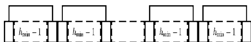
FIG. 10. Principle of a nondesignable structure. Structures consisting of a repeated pattern of simple paired bases become undesignable, if this pattern is repeated often enough. For results see Table I.
